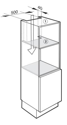
To ensure that the Combi Steam Oven has adequate ventilation, the following cut-outs measuring  $19 \ 11/16" \times 1 \ 9/16"$  (500 x 40 mm) must be made:
